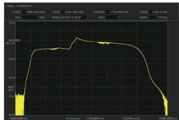
Measurement example of 2 \mu\text{m} supercontinuum light source (by use of Extended model)
