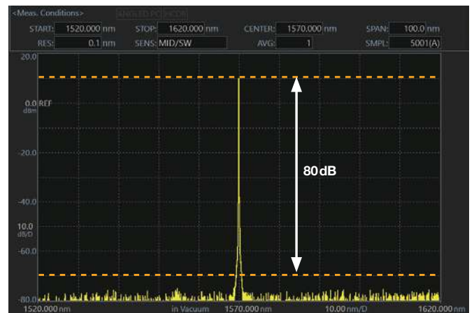
AQ6370E, Sensitivity setting: MID High dynamic mode: ON, typical
